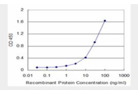
Detection limit for recombinant GST tagged CSTB is approximately 1ng/ml as a capture antibody.
