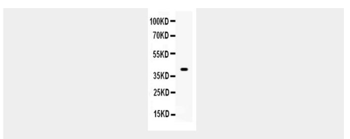
Anti- WNT1 Picoband antibody, ABO12149, Western blottingAll lanes: Anti WNT1 (ABO12149) at 0.5ug/mlWB: COLO320 Whole Cell Lysate at 40ugPredicted bind size: 41KDObserved bind size: 41KD
