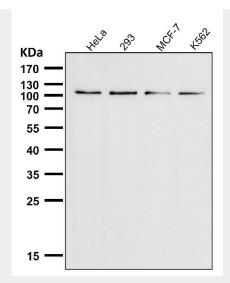
All lanes use the Antibody at 1:3K dilution for 1 hour at room temperature.
