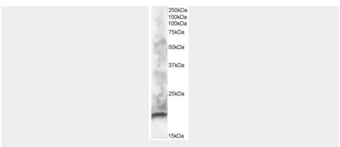
AF1174a staining (1  $\mu$ g/ml) of human brain lysate (RIPA buffer, 30  $\mu$ g total protein per lane). Primary incubated for 1 hour. Detected by western blot using chemiluminescence.
