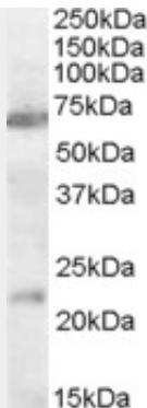
AF1239a (0.3 µg/ml) staining of Rat Brain lysate (35 µg protein in RIPA buffer). Primary incubation was 1 hour. Detected by chemiluminescence.
