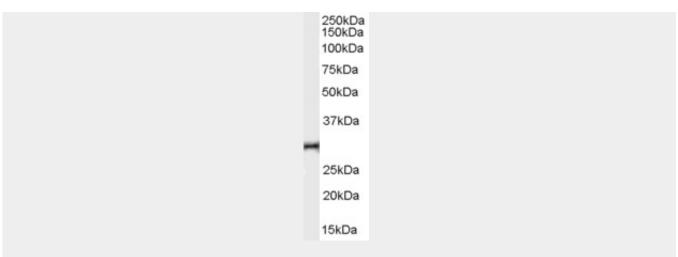
AF1547a (0.03  $\mu$ g/ml) staining of human thymus lysate (35  $\mu$ g protein in RIPA buffer). Primary incubation was 1 hour. Detected by chemiluminescence.
