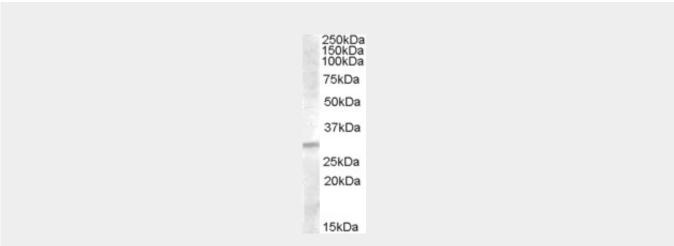
AF1558a (1  $\mu$ g/ml) staining of Human Liver lysate (35  $\mu$ g protein in RIPA buffer). Primary incubation was 1 hour. Detected by chemiluminescence.
