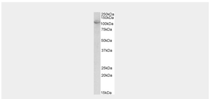
AF4078a (2  $\mu$ g/ml) staining of A431 lysate (35  $\mu$ g protein in RIPA buffer). Primary incubation was 1 hour. Detected by chemiluminescence.
