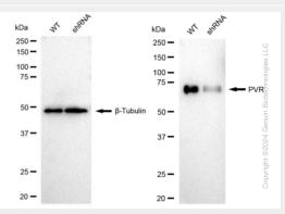
Western blotting analysis using anti-PVR antibody (Cat#AGI1276). PVR expression in wild type (WT) and PVR shRNA knockdown (KD) HeLa cells with 30  $\mu$ g of total cell lysates.  $\beta$ -Tubulin serves as a loading control. The blot was incubated with anti-PVR antibody (Cat#AGI1276, 1:5,000) and HRP-conjugated goat anti-rabbit secondary antibody respectively.
