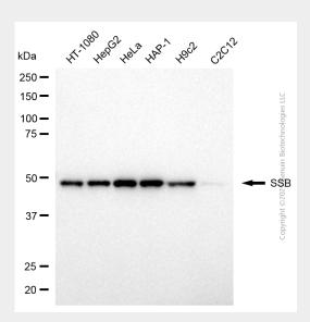
Western blotting analysis using anti-SSB antibody (Cat#AGI2073). Total cell lysates (30  $\mu$ g for H9c2 and C2C12, 10  $\mu$ g for others) from various cell lines were loaded and separated by SDS-PAGE. The blot was incubated with anti-SSB antibody (Cat#AGI2073, 1:2,500) and HRP-conjugated goat anti-mouse secondary antibody respectively.
