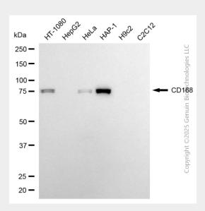
Western blotting analysis using anti-CD168 antibody (Cat#AGI2100). Total cell lysates (30  $\mu$ g) from various cell lines were loaded and separated by SDS-PAGE. The blot was incubated with anti-CD168 antibody (Cat#AGI2100, 1:5,000) and HRP-conjugated goat anti-rabbit secondary antibody respectively.
