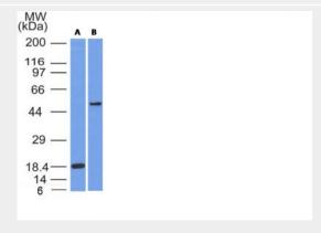
Western Blot of SOX10(A) Recombinant protein (B) A375 Cell Lysateusing SOX10 Monoclonal Antibody (SOX10/991 + SOX10/1074).
