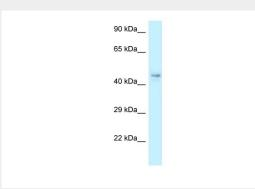
WB Suggested Anti-Cops4 Antibody Titration: 1.0  $\mu\text{g/ml}$  Positive Control: Rat Lung
