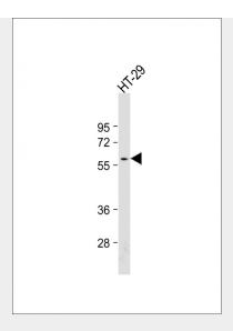
Anti-SRC Antibody at 1:500 dilution + HT-29 whole cell lysate Lysates/proteins at 20  $\mu$ g per lane. Secondary Goat Anti-Mouse IgG, (H+L), Peroxidase conjugated at 1/10000 dilution. Predicted band size : 60 kDa Blocking/Dilution buffer: 5% NFDM/TBST.
