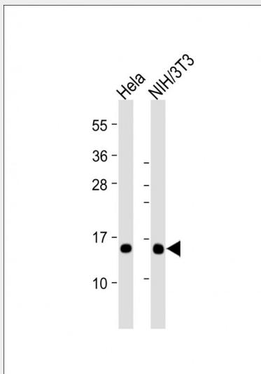
All lanes : Anti-RBX1 at 1:2000 dilution Lane 1: HeLa whole cell lysate Lane 2: NIH/3T3 whole cell lysate Lysates/proteins at 20 µg per lane. Secondary Goat Anti-mouse IgG, (H+L), Peroxidase conjugated at 1/10000 dilution. Predicted band size : 12 kDa Blocking/Dilution buffer: 5% NFDM/TBST.
