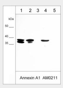
Western blot of human A431 cells (lane 1), A549 cells (lane 2), LNCaP cells (lane 3), full-length recombinant human annexin A1 (lane 4), and recombinant human annexin A2 (lane 5). The blot was probed with mouse monoclonal anti-Annexin A1 antibody (AM0211) at 1:1000 (lanes 1-5).
