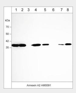
Western blot of human A431 (lane 1), MDA-MB-231 (lane 2), LNCaP (lane 3), MeWo (lane 4), HUVEC (lane 5), Jurkat (lane 6), K562 (lane 7), and PC3 (lane 8) cell lysates. The blot was probed with mouse monoclonal anti-Annexin A2 antibody (AM0091) at 1:500 (lanes 1-8).
