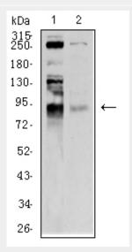
Western blot analysis using BRD2 mouse mAb against C6 (1) and Hela (2) cell lysate.
