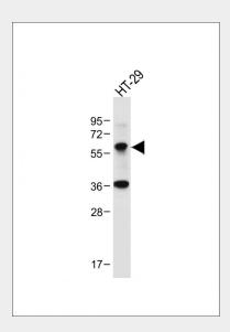
Anti-hChk1-S280 at 1:1000 dilution + HT-29 whole cell lysate Lysates/proteins at 20  $\mu$ g per lane. Secondary Goat Anti-Rabbit lgG, (H+L), Peroxidase conjugated at 1/10000 dilution. Predicted band size : 54 kDa Blocking/Dilution buffer: 5% NFDM/TBST.
