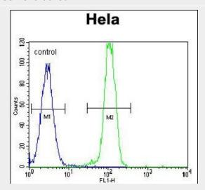
B2M Antibody (C-term) (Cat. #AP2771b) flow cytometric analysis of Hela cells (right histogram) compared to a negative control cell (left histogram).FITC-conjugated goat-anti-rabbit secondary antibodies were used for the analysis.
