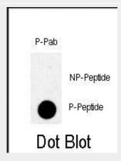
Dot blot analysis of anti-Phospho-TBK-pS172 Antibody (Cat.#AP3627a) on nitrocellulose membrane. 50ng of Phospho-peptide or Non Phospho-peptide per dot were adsorbed. Antibody working concentrations are 0.5ug per ml.
