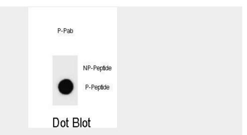
Dot blot analysis of Phospho-KIT-S746 Antibody Phospho-specific Pab (Cat. #AP3784b) on nitrocellulose membrane. 50ng of Phospho-peptide or Non Phospho-peptide per dot were adsorbed. Antibody working concentrations are 0.6ug per ml.
