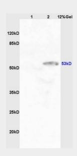
Lane 1: mouse kidney lysates Lane 2: human kidney lysates probed with Anti CYP11A1/P450SCC Polyclonal Antibody, Unconjugated (AP52081) at 1:200 in 4°C. Followed by conjugation to secondary antibody at 1:3000 90min in 37°C. Predicted band 53/57kD. Observed band size: 53kD.
