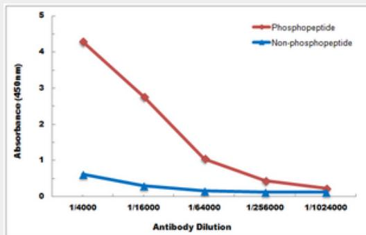
Direct ELISA antibody dose-response curve using Anti-CHK1 (pS345) Antibody. Antigen (phosphopeptide and non-phosphopeptide) concentration is 5 ug/ml. Goat Anti-Rabbit IgG (H&L) - HRP was used as the secondary antibody, and signal was developed by TMB substrate.
