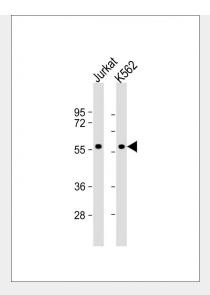
All lanes : Anti-MEF2C Antibody (S396) at 1:1000 dilution Lane 1: Jurkat whole cell lysate Lane 2: K562 whole cell lysate Lysates/proteins at 20  $\mu$ g per lane. Secondary Goat Anti-Rabbit IgG, (H+L), Peroxidase conjugated at 1/10000 dilution. Predicted band size : 51 kDa Blocking/Dilution buffer: 5% NFDM/TBST.
