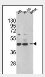
Western blot analysis of HSD17B7 Antibody (N-term) (Cat. #AP6760a) in 293,HL-60,Jurkat cell line lysates (35ug/lane). HSD17B7 (arrow) was detected using the purified Pab.(2ug/ml)
