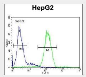
SERPINH1 Antibody (Center) (Cat. #AP7366c) flow cytometric analysis of HepG2 cells (right histogram) compared to a negative control cell (left histogram).FITC-conjugated goat-anti-rabbit secondary antibodies were used for the analysis.
