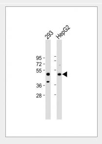
All lanes : Anti-MAPK8 Antibody (C-term) at 1:2000 dilution Lane 1: 293 whole cell lysate Lane 2: HepG2 whole cell lysate Lysates/proteins at 20  $\mu$ g per lane. Secondary Goat Anti-Rabbit lgG, (H+L), Peroxidase conjugated at 1/10000 dilution. Predicted band size : 48 kDa Blocking/Dilution buffer: 5% NFDM/TBST.
