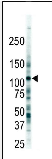
Western blot analysis of anti-FLT3 Pab (Cat. #AP7644b) in 293 cell lysate. FLT3 (arrow) was detected using purified Pab. Secondary HRP-anti-rabbit was used for signal visualization with chemiluminescence.
