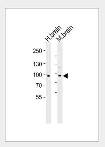
Western blot analysis of lysates from human brain and mouse brain tissue lysate(from left to right), using CDH20 Antibody (N-term)(Cat. #AP9870a). AP9870a was diluted at 1:1000 at each lane. A goat anti-rabbit IgG H&L(HRP) at 1:5000 dilution was used as the secondary antibody. Lysates at 35ug per lane.
