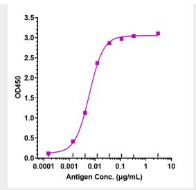
Immobilized human IL-18 His at4  $\mu$ g/mL can bind Anti-PTPRC / CD45 Reference Antibody (Novartis patent anti-CD45) $\square$ EC50=0.00604  $\mu$ g/mL.
