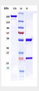
Anti-CDCP1 / CD318 Reference Antibody (38 E11) on SDS-PAGE under reducing (R) condition. The gel was stained with Coomassie Blue. The purity of the protein is greater than 95%
