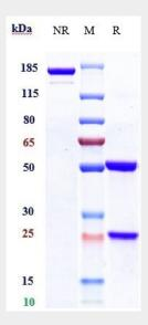
Anti-HGFR / c-Met Reference Antibody (telisotuzumab) on SDS-PAGE under reducing (R) condition. The gel was stained with Coomassie Blue. The purity of the protein is greater than 95%
