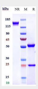
Anti-FGFR4 / CD334 Reference Antibody (U3-1784) on SDS-PAGE under reducing (R) condition. The gel was stained with Coomassie Blue. The purity of the protein is greater than 95%
