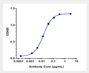
Immobilized human CSF1R / M CSFR, Fc tag at 2  $\mu$ g/mL can bind Anti-CSF1R / M-CSFR / CD115 Reference Antibody (cabiralizumab) $\square$ EC50=0.01383  $\mu$ g/mL
