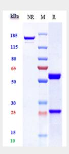
Anti-ERBB3 / HER3 Reference Antibody (barecetamab) on SDS-PAGE under reducing (R) condition. The gel was stained with Coomassie Blue. The purity of the protein is greater than 95%
