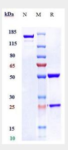
Anti-F3 / Factor III / Tissue Factor / CD142 Reference Antibody (tisotumab) on SDS-PAGE under reducing (R) condition. The gel was stained with Coomassie Blue. The purity of the protein is greater than 95%
