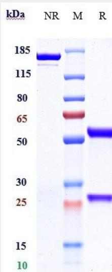
Anti-ERBB1 / EGFR / HER1 Reference Antibody (cetuximab) on SDS-PAGE under reducing (R) condition. The gel was stained with Coomassie Blue. The purity of the protein is greater than 95%
