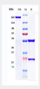
Anti-HGFR / c-Met Reference Antibody (Metheresis patent anti-Met) on SDS-PAGE under reducing (R) condition. The gel was stained with Coomassie Blue. The purity of the protein is greater than 90%
