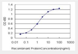
Detection limit for recombinant GST tagged EXOC4 is approximately 0.1ng/ml as a capture antibody.
