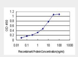
Detection limit for recombinant GST tagged GPS1 is approximately 1ng/ml as a capture antibody.
