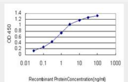
Detection limit for recombinant GST tagged MCPH1 is approximately 0.03ng/ml as a capture antibody.
