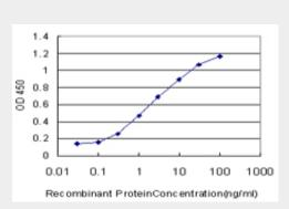
Detection limit for recombinant GST tagged SCARB2 is approximately 0.1ng/ml as a capture antibody.
