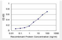
Detection limit for recombinant GST tagged UBTF is approximately 1ng/ml as a capture antibody. UBTF Antibody (monoclonal) (M04) - Background
