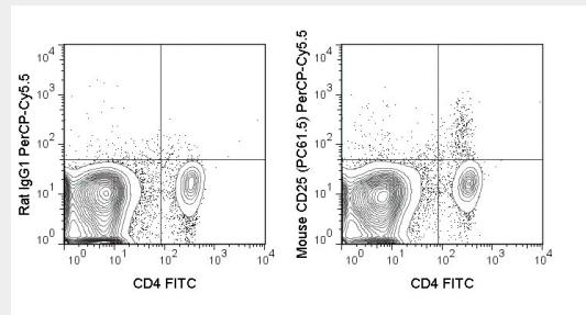
C57Bl/6 splenocytes were stained with FITC Anti-Mouse CD4 (35-0041) and 0.25 ug PerCP-Cy5.5 Anti-Mouse CD25 (ATB10272) (right panel) or 0.25 ug PerCP-Cy5.5 Rat IgG1 (left panel).
